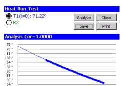
... also temperature of winding at time "0" can be extrapolated and shown.
