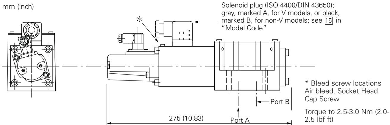
**Note:** For optimum valve operation, bleed the air from the proportional solenoids at initial start-up. This may be done as follows:
