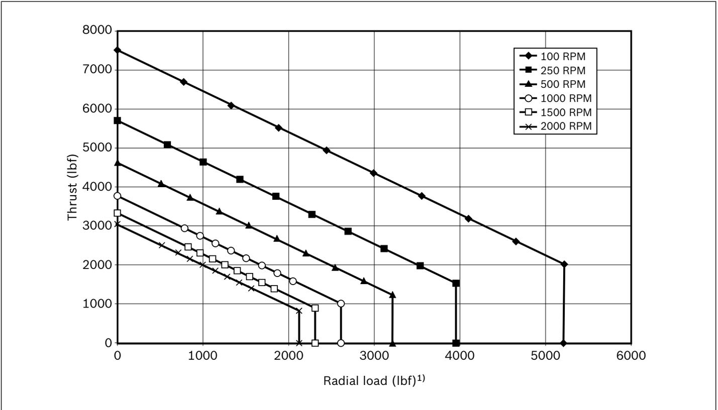
1) Radial load located at center of effective output of the shaft.
