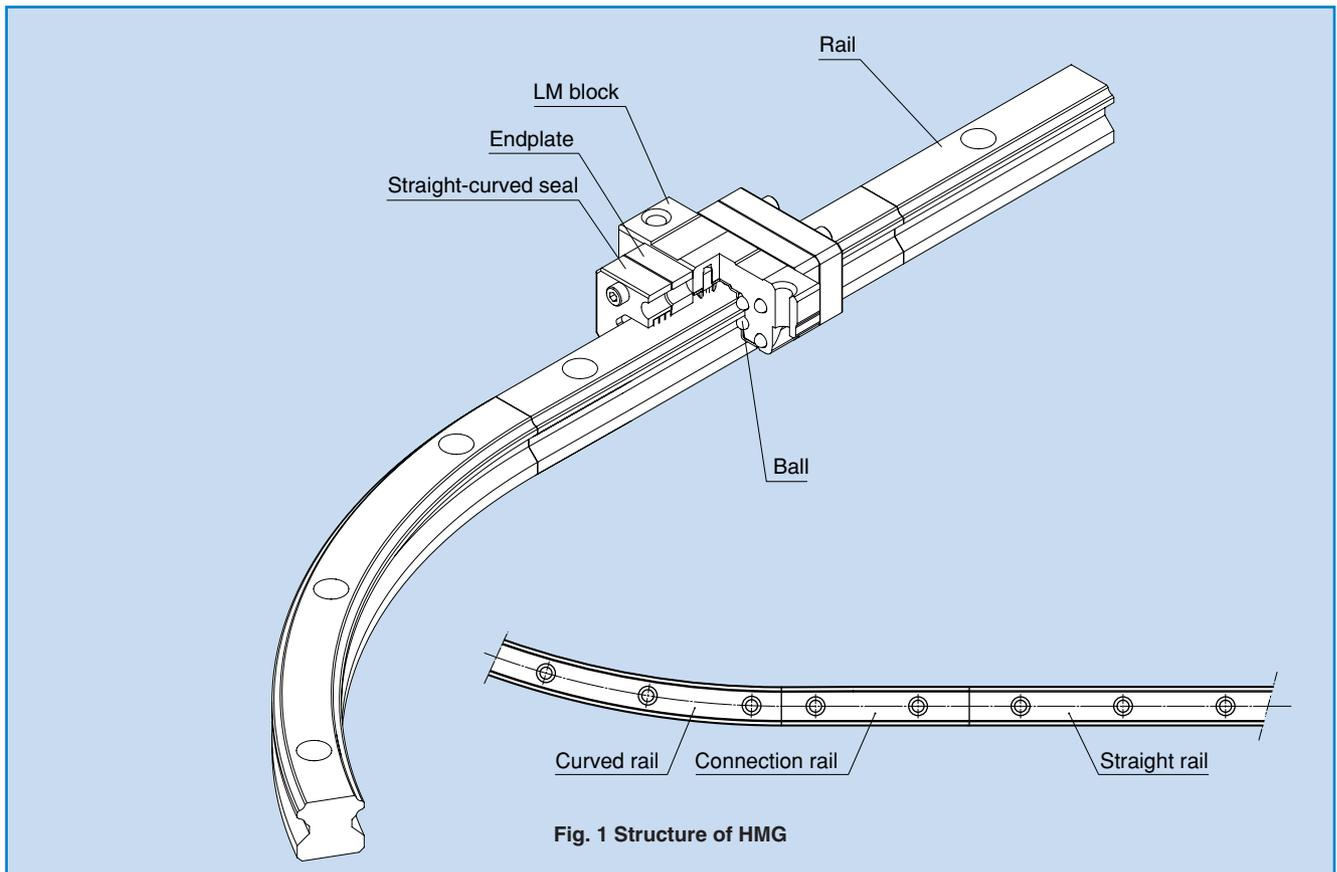
The Straight-Curved Guide HMG is a new straight-curved guide that allows the same type of LM blocks to continuously move on straight and curved rails by combining the technologies of the LM Guide HSR and the R Guide HCR. It achieves drastic cost reduction through improvement of work efficiency at the assembly and conveyance lines and the inspection equipment and simplification of the structure by eliminating a lift and a table.
