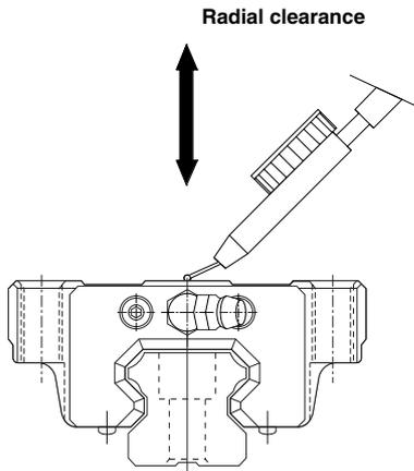
In general, selecting a negative clearance (i.e., a preload\*1 is applied) while taking into account possible vibrations and impact generated from reciprocating motion favorably affects the service life and the accuracy.
