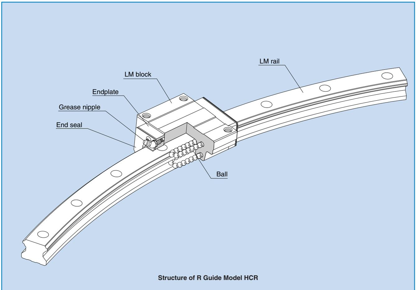
Balls roll in four rows of raceways precision-ground on an LM rail and an LM block, and endplates incorporated in the LM block allow the balls to circulate.
