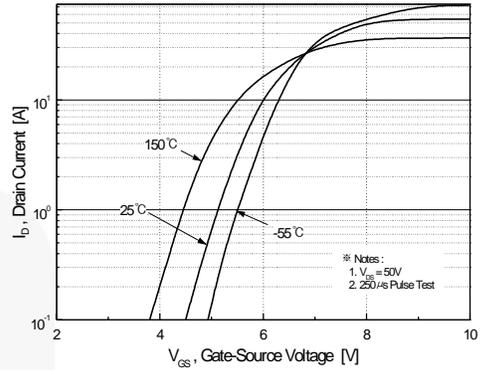
**Figure 2. Transfer Characteristics**
