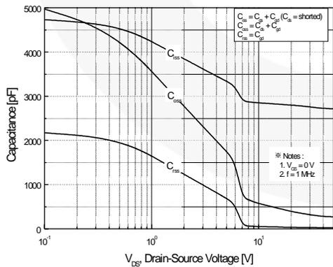
**Figure 5. Capacitance Characteristics**
