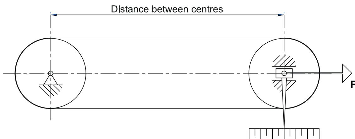
The effective length is verified placing the belt on two equal pulleys having same groove profile. The specified measuring tension F is applied to the shaft of one pulley.
