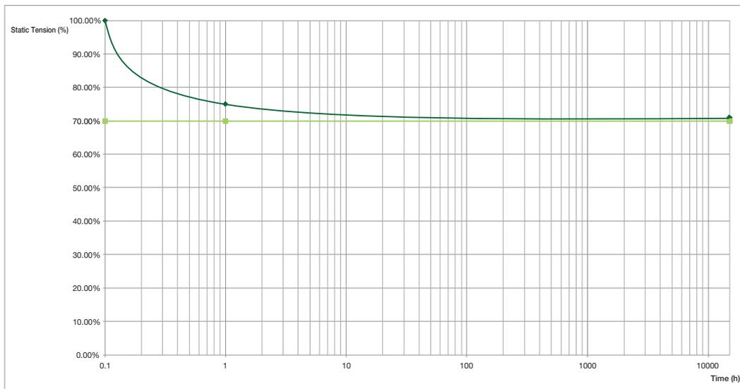
Under normal conditions, static tension fall is quite fast (some minutes). After this initial fall the static tension is stable. Please note that this fall is fairly high (30% - 40% than the initial static load).
