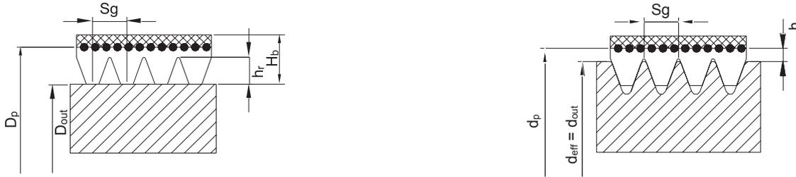
**D<sub>p</sub>**: The pitch diameter is used to calculate the transmission ratio and the belt speed.
