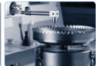
Computerized mapping of gear tooth profile
