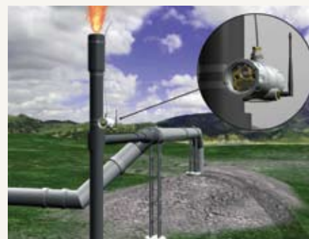
Flare Stack Ignition Verification
