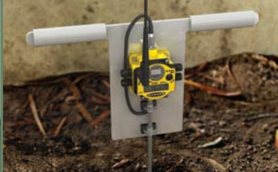
Compost Temperature Monitoring
