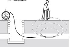
Note: The blade of the locator must be in line with the sonde, the opposite to cable locating.
