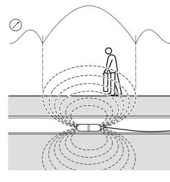
It is a good idea to locate the ghosts as finding them positively confirms the position of the main peak. To lose the ghosts subsequently, reduce the sensitivity of the locator a little to leave only the main peak detectable.
