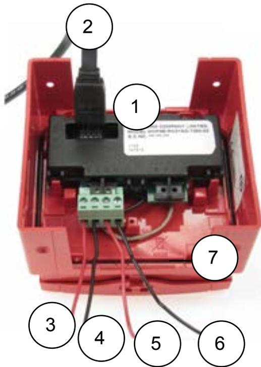
The FC421CP-I has a factory set (invalid) address of 255. The FC421CP-I is field programmed with the address prior to installation using a FireClass address programming tool. The associated ancillary programming lead plugs into the programming port. Ensure that the pins of the ancillary programming lead are inserted completely into the lower row of the programming port for effective communication with the address programming tool.
