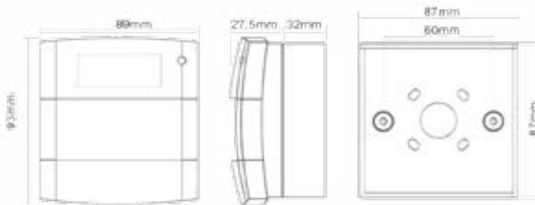
The FC420CP-I may be fitted to a standard (surface mounting) call point back box which is available separately.
