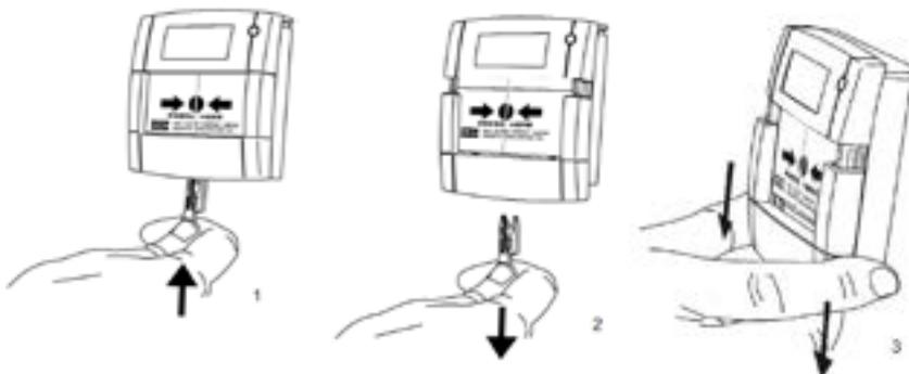
A test key is provided with each MCP to allow easy testing of the switch mechanism and wiring, without breaking the frangible element. The key is inserted into a slot in the base of the MCP, allowing the frangible element to drop away from the switch, thus activating it and registering an alarm at the CIE. Note: the key should not be left with the MCP after commissioning, but may be left inside the CIE for convenience.
