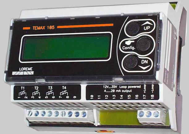
TEMAX105LCD is a 4-20mA loop powered digital transmitter with LCD display allowing signal processing of Pt100 temperature sensors (maximum value, minimum value, average value).
