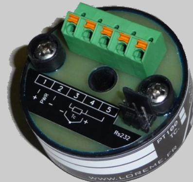
The CNL40ig is a universal smart in-head mounting temperature sensor transmitters. Cover all temperature measurement (RTD and thermocouples) in all range with an unique device. The CNL40igH integrate the HART communication protocol, FDT compliant and it is available with SIL2 conformity according to IEC 61508 standard.
