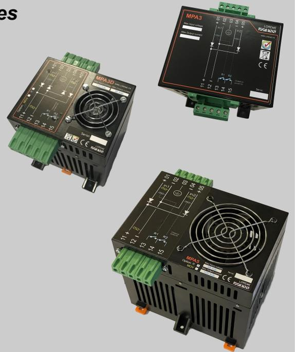
The redundant module provide an effective protection against the power supplies failure. Through decoupling of two power supplies, the failure of one of them has no effect on the output, the other taking automatically its function without interruption. The redundant module monitor continuously the two power supplies, and provide an alarm via a contact relay if a failure is detected (loss of redundancy).
