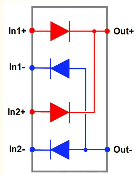
**WIRING AND OUTLINE DIMENSIONS: MPA3D dual circuit common Cathode and common Anode**
