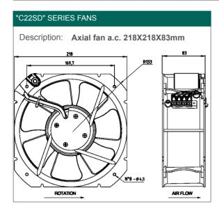
Impeller material: fibre reinforced plastic (PA66) blades
