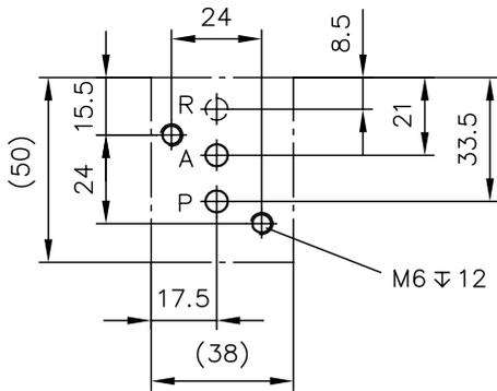
The hole pattern corresponds to that of type ADM 11 P as per [D 7120](#). The O-ring counterbore for the drain port R (or L) is present but is only required for type CDK...-SP.
