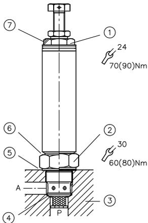
1. Before screwing in the valve, loosen the lock nut and sealing nut until the travel stop.
