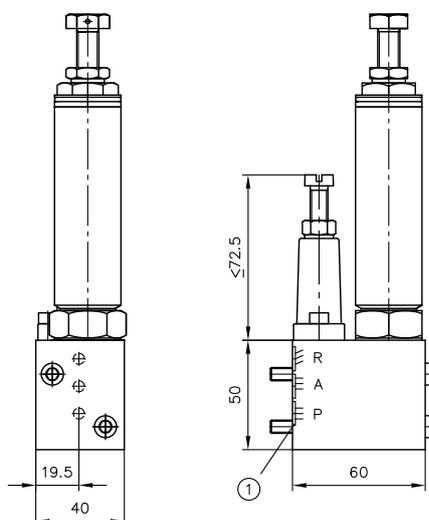
1 Sealing with O-rings 7.65x1.78 NBR 90 Sh
