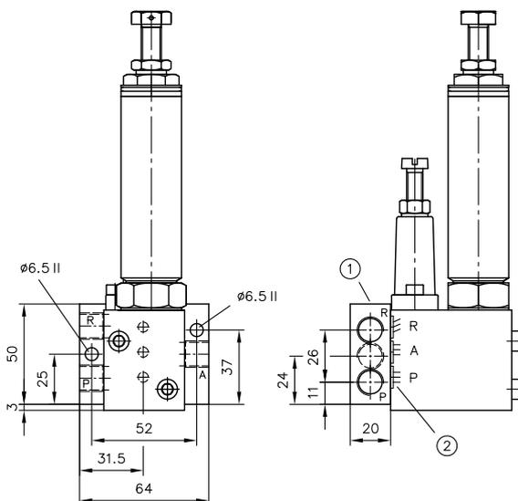
1 Adapter plate (connection block for pipe connection)
