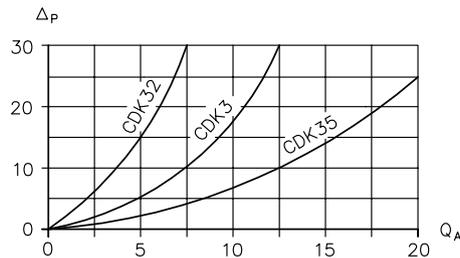
$Q_A$  Volumetric flow rate (lpm);  $\Delta p$  Flow resistance (bar)
