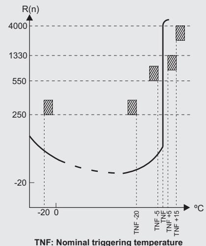
Characteristics of PTC thermistor probe as per standard DIN 44081 (or IEC 34-11)
