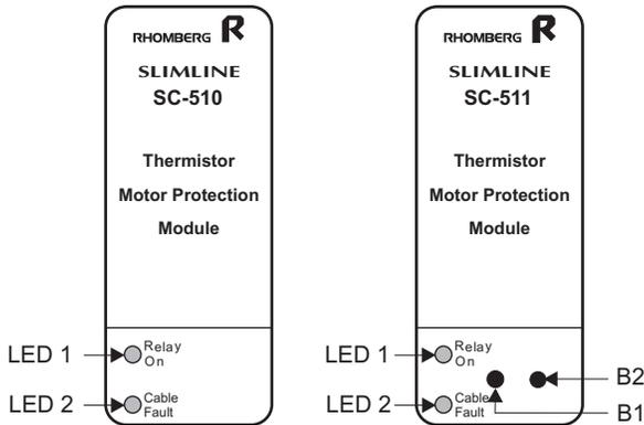
LED1: The LED marked “Relay ON” illuminates when the relay is energised.
